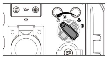
**Important:** Always ensure that the EZ Start dial and fuel lever vent are in the "STOP" and "OFF" position, respectively, position when the generator is not in use.
