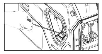
As engine warms up, push the choke knob in to the "RUN" position.
