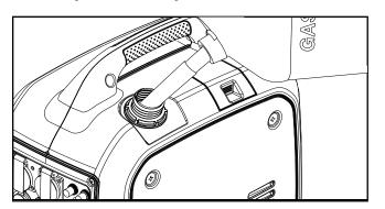
3. Screw on the gasoline cap until you hear a "clicking" noise. Wipe up any spilled fuel.
