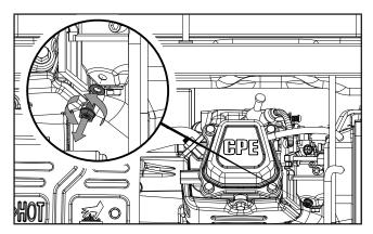
5d. When petrol stops flowing from the carburetor, replace and tighten the carburetor drain bolt and be sure to properly dispose of the drained petrol according to local regulations or guidelines.
