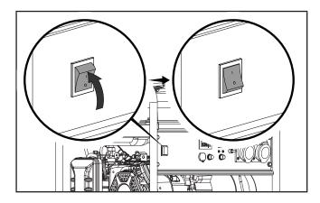
Move the choke to the CHOKE position. Note: for restarting a warm engine, move the choke to 75% of the CHOKE position.
