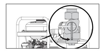
Push the engine switch to the "ON" position.
