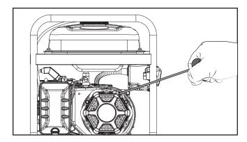
7. As soon as engine starts, move the choke to the "RUN" position over a 2-5 second duration.
